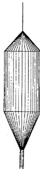
Fig. 2: Antennas were Guarini's speciality and this is the design used in conjunction with the 'first repeater' (see text).
